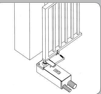
Remove the plug, insert the box wrench into the gate lever and turn in the indicated direction.
